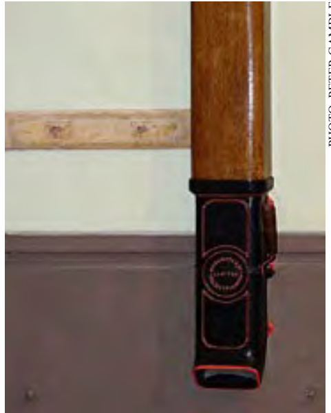
DETAIL SHOWING GRAIN CONTROL OUTLET - RESTORED BY ROGER BLAKE
